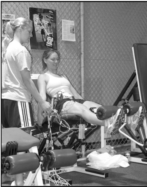
Figure 3. A piece of commercial exercise equipment for exercising the quadriceps muscles is shown. EMG electrodes are attached to the quadriceps, abdominal muscles, and other muscle groups to assess muscle use during exercise at various levels of weight lifting.
