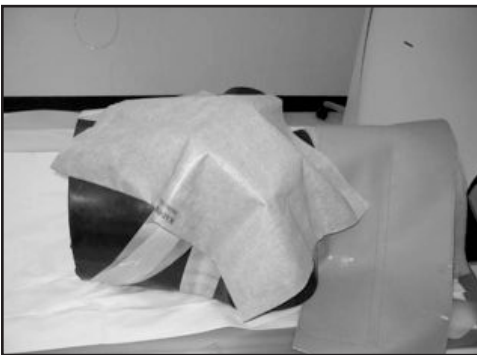
Figure 2. Tungsten-antimony composite breast shield (RADPAD; Worldwide Innovations & Technologies, Inc., Overland Park, Kansas) draped over the combination breast tissue equivalent and anthropomorphic adult head and torso phantom.
